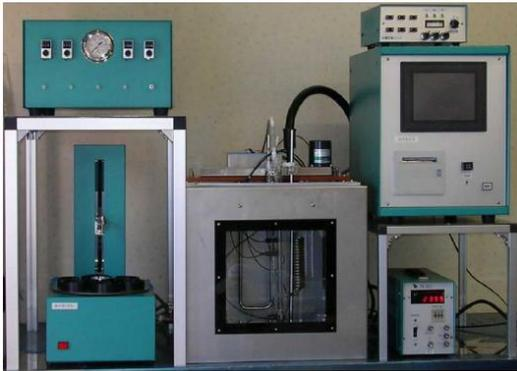
Figure 1: Automatic viscometer DT-553
