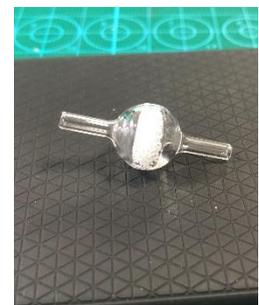
Figure 7: Contamination prevention filter
