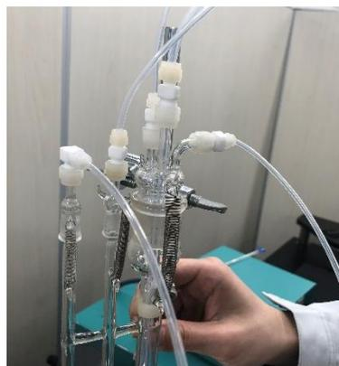
Figure 6: Upper part of viscosity tube
